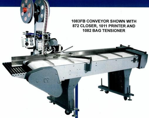
The Kwik Lok 1083 Belt Conveyor will handle packages up to 20" (45 cm) in length at speeds of 60 or 90 packages per minute. Faster speeds and a kit to widen the conveyor (for packages in excess of 20" (45 cm) can be furnished. The conveyor can also be ordered with a brake-clutch unit that provides bag actuation. Conveyor lengths of 7.5' (2.29m) to 30' (9.1 m) are available.
